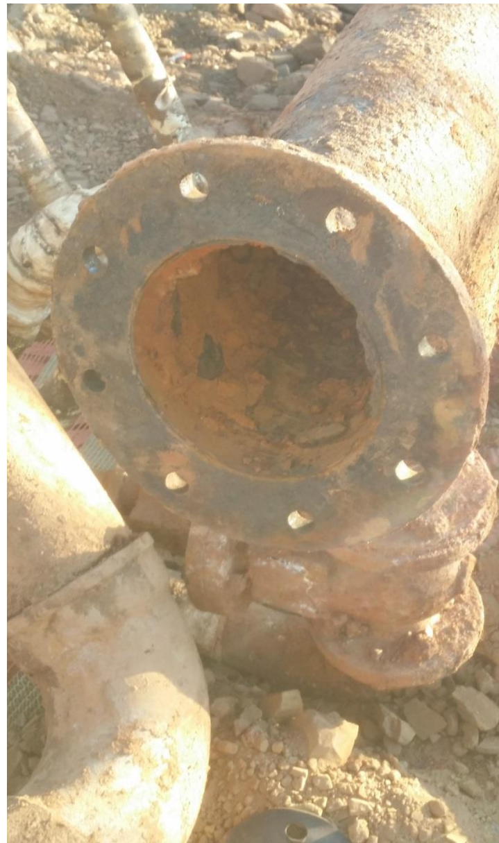
Old water meters being removed. Note the condition of the pipe below
